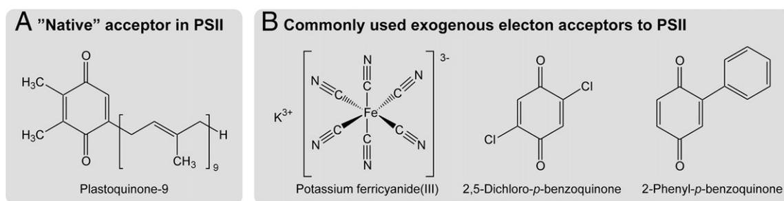
Fig. 1. Structures of the electron acceptors to PSII membrane fragments used in this study.
